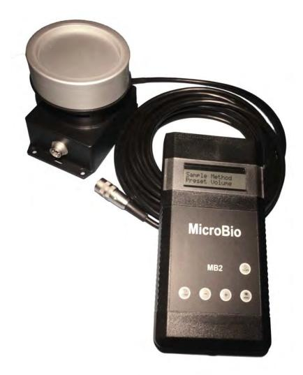
The first task is to run the connecting cable from where the sampling head is to be positioned to where the control unit is to be located.
