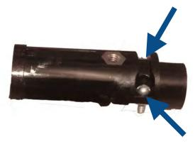
4. Solder cable onto connector pins. The connector body has pin numbers embossed onto the surface adjacent to the pins.
