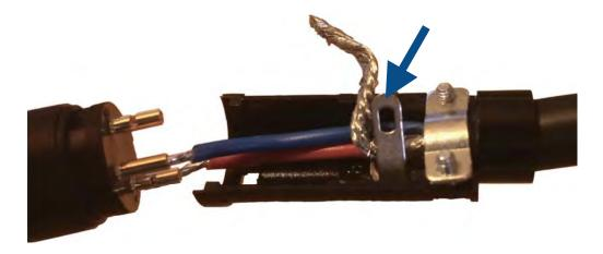
6. Fit the pin housing back onto the frame, noting the raised pegs on the rim of the pin housing that sit into the holes on the frame. Then replace the frame cover.
