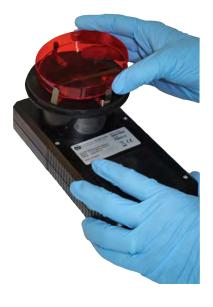
The standard MicroBio MB2 can use 220 or 400 hole sampling heads. The 220 hole sampling head can be used with both 55mm/65mm contact plates or 90mm petri dishes, but only the centre 55mm of the petri dish will collect samples. Using the 400 x 0.7mm hole sampling head will give nearly full coverage of a 90mm petri dish, improving reliability of counts.
