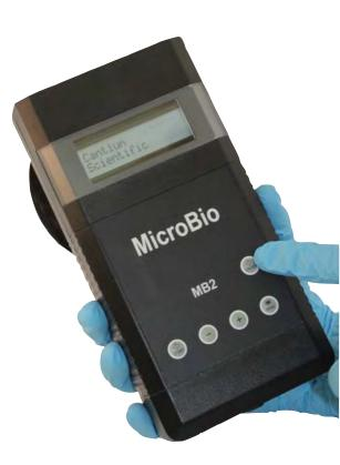
If the battery is too low, the MicroBio MB2 will issue a warning to change the battery and then automatically switch off. This is to protect the battery pack and not allow samples to be taken that may not complete.
