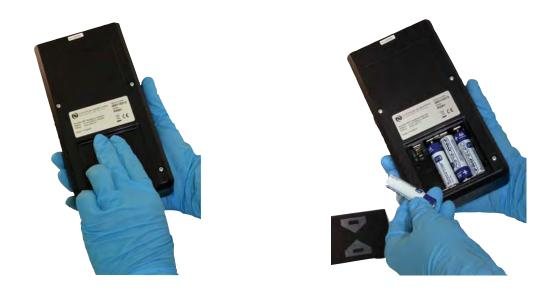
The orientation of the cells is indicated within the battery compartment.
