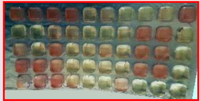
Pseudocult P/A Broth converted to MPN count in 100-250 mL drinking or bath water: Pseudomonas aeruginosa positive wells are distinctly pink, not just fluorescent
