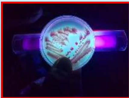
Rapid Pseudomonas Agar (CN ISO 16266 with chromogen) for confirmative detection and enumeration of P. aeruginosa in just 18h: red colonies with subsequent fluorescence
