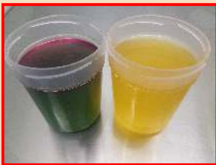
Colicult-Plus ISO 9308-2 with additional chromogen: negative screening for E. coli (turning green without misinterpretation of fluorescence, and red indole) and rest of coliforms (turning yellow) in 100-250 mL of drinking or bath water
